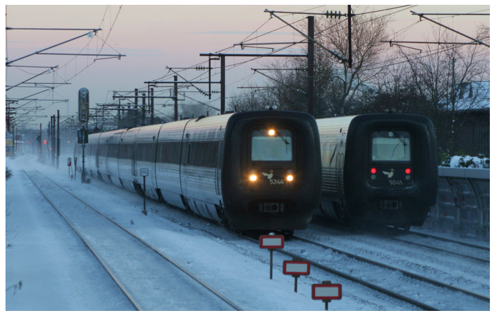
Two IC3 trains pass Rødover, about 7 km west of Copenhagen Central station on 10 December 2010. The markers announce a main signal in 400m. Photo Finn Møller.
